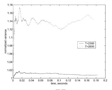
**FIG. 14.** The normalized variance  $(\overline{u_m^2}/u_m^2)$  of the mean enclosure volumes of each droplet at different temperatures.
