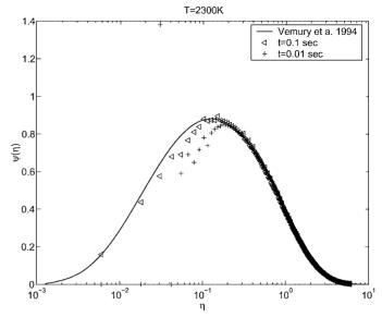
**FIG. 12.** The enclosure size distribution at T = 2300 K. Dimensionless number density,  $\psi(\eta) = \frac{n(u,t)\bar{u}}{n^{\infty}}$  versus dimensionless volume,  $\eta = u/\bar{u}$ . The numerical values of the self-preserving distribution for the Brownian regime (solid line) is taken from Vemury *et al.* (24).
