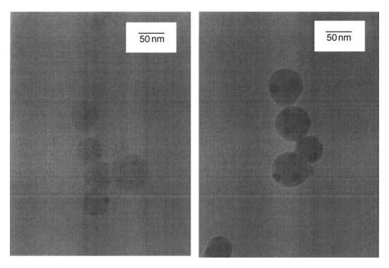
FIG. 2. Evolution of the aerosol (SiO<sub>2</sub>) and minor phase (Fe<sub>2</sub>O<sub>3</sub>) during the growth of SiO<sub>2</sub>/Fe<sub>2</sub>O<sub>3</sub> nanocomposites.
