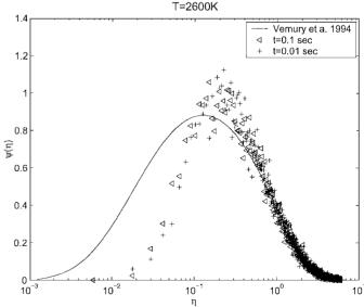
**FIG. 13.** The enclosure size distribution at T = 2600 K. Dimensionless number density,  $\psi(\eta) = \frac{n(u,t)\bar{u}}{n^{\infty}}$  versus dimensionless volume,  $\eta = u/\bar{u}$ . The numerical values of the self-preserving distribution for the Brownian regime (solid line) is taken from Vemury *et al.* (24).
