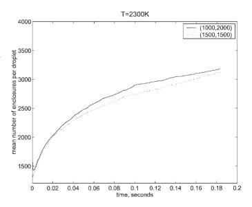
FIG. 4. Mean number of the enclosures per droplet (total number of enclosures/total number of droplets) at T = 2300 K for two values of (M, m), where *M* refers to the initial number of droplets and *m* refers to the initial number of enclosures per droplet in our simulation. All droplets and enclosures are initially monodisperse.
