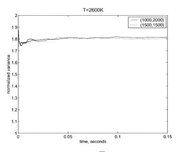
FIG. 9. Normalized second moment  $(\overline{u^2}/\overline{u^2})$  of the enclosures at T =2600 K for two values of (M, m).
