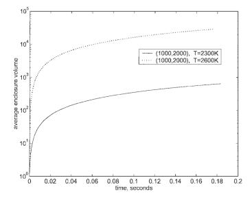
FIG. 11. Comparison of the average volume of the enclosures at T = 2300 K and T = 2600 K. Note a log scale along the vertical axis.
