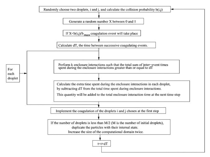
FIG. 3. Flow chart of the hybrid Monte Carlo algorithm.
