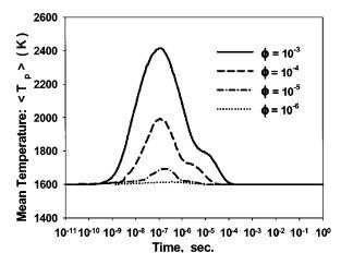
FIG. 17. The effect of different particle volume loading ( $\phi = 10^{-3}, 10^{-4}, 10^{-5}, 10^{-6}$ ) on the temporal variation of mean particle temperature ( $\langle T_p \rangle$ ),  $T_g = 1600$  K and gas pressure,  $P_g = 101$  kPa (1 atm) for titania nanoparticle coalescence.
