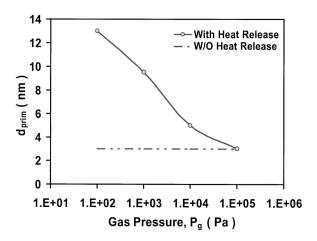
FIG. 10. The effect of background gas pressures  $(P_g)$  on primary particle size  $(d_{\text{prim}})$  for silicon nanoparticles at constant gas temperature,  $T_g = 500 \text{ K}$  and particle volume loading,  $\phi = 10^{-6}$ . The primary particle size predicted without a heat release effect has also been indicated.
