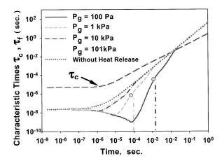
FIG. 8. Variation of characteristic coalescence/fusion ( $\tau_f$ ) and characteristic collision ( $\tau_c$ ) times with residence time for various background gas pressures,  $P_g$ ,  $T_g$ = 500 K and particle volume loading,  $\phi$ =  $10^{-6}$ . A gray point marks the gradient change for  $\tau_f$  corresponding to the point where  $A/A_{\rm sph} \geqslant 1$ . Results are for silicon.
