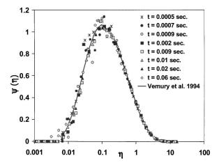
FIG. 4. Self-preserving size distribution for coagulation from the Monte Carlo method compared with the numerical results of Vemury *et al.* (Ref. 43) and plotted as the dimensionless number density,  $\psi(\eta) = N(t,V_p) \bar{V}_p / N_\infty$  versus dimensionless volume,  $\eta = V_p / \bar{V}_p$ . Silicon at  $T_g = 320$  K was considered assuming a free molecular regime collision kernel.
