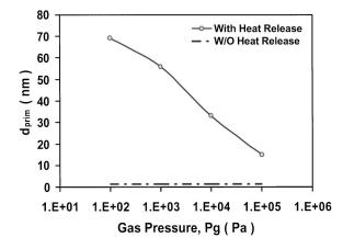
FIG. 14. The effect of background gas pressures  $(P_g)$  on primary particle sizes  $(d_{\text{prim}})$  for titania nanoparticle coalescence at  $T_g$  = 1600 K, and particle volume loading,  $\phi$  = 10<sup>-3</sup>. Primary particle size without the heat release effect has also been indicated.
