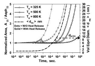
FIG. 7. Variation of silicon normalized area and mean volume equivalent diameter with residence time for various background gas temperatures,  $T_g$ ,  $P_g = 100$  Pa, and particle volume loading,  $\phi = 10^{-6}$  ( $A_{(i)}$ : particle area and  $A_{\text{sph(i)}}$ : equivalent spherical area of the corresponding particle).
