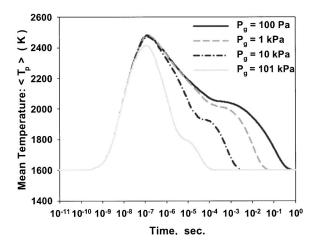
FIG. 13. The variation of the mean particle temperature ( $\langle T_p \rangle$ ) with residence time for various background gas pressures,  $P_g$ ,  $T_g$ =1600 K, and particle volume loading,  $\phi$ =10<sup>-3</sup> for titania nanoparticle coalescence.
