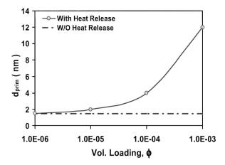
FIG. 18. The effect of particle volume loading ( $\phi = 10^{-3}, 10^{-4}, 10^{-5}, 10^{-6}$ ) on the prediction of primary particle sizes ( $d_{\text{prim}}$ ) for titania nanoparticle coalescence,  $T_g = 1600 \text{ K}$ , and gas pressure,  $P_g = 101 \text{ kPa}$  (1 atm). A primary particle size without heat release effect has also been indicated.
