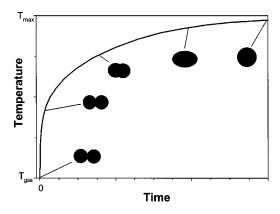
FIG. 1. Schematic representation of the temporal evolution of particle temperature and shape in the nanoparticle coalescence process.
