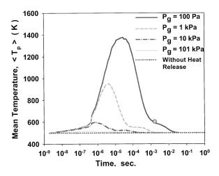
FIG. 9. The variation of mean silicon particle temperature ( $\langle T_p \rangle$ ) with residence time for various background gas pressures,  $P_g$ ,  $T_g$ =500 K, and particle volume loading,  $\phi$ =10<sup>-6</sup>. A gray point marks the gradient change for  $\tau_f$  corresponding to the point where  $A_{(i)}/A_{\text{sph}(i)} \geqslant 1$ .
