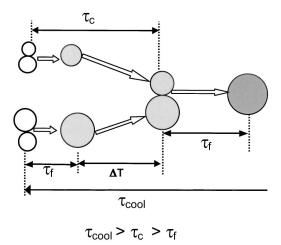
FIG. 2. The schematic diagram indicating the various time scales; mean interevent time ( $\Delta T$ ), characteristic coalescence/fusion ( $\tau_c$ ), characteristic collision ( $\tau_c$ ), and the mean cooling time for particles ( $\tau_{\rm cool}$ ).
