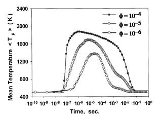
FIG. 15. The effect of different particle volume loading ( $\phi = 10^{-4}, 10^{-5}, 10^{-6}$ ) on the temporal variation of the mean particle temperature ( $\langle T_p \rangle$ ) at constant gas temperature  $T_g = 500 \, \mathrm{K}$  and gas pressure  $P_g = 100 \, \mathrm{Pa}$  for silicon particle coalescence.
