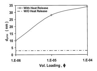
FIG. 16. The effect of particle volume loading ( $\phi = 10^{-4}, 10^{-5}, 10^{-6}$ ) on the prediction of primary particle sizes ( $d_{\text{prim}}$ ) for silicon nanoparticle coalescence  $T_g = 500 \text{ K}$  and gas pressure,  $P_g = 100 \text{ Pa}$ . Primary particle size predicted without heat release effect has also been indicated.
