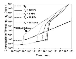
FIG. 11. The variation of characteristic fusion  $(\tau_f)$  and characteristic collision  $(\tau_c)$  times with residence time in titania nanoparticle coalescence for various background gas pressures,  $P_g$ ,  $T_g = 1600$  K, and particle volume loading,  $\phi = 10^{-3}$ . An open circle indicates an abrupt change in the gradient of  $\tau_f$  corresponding to the phase change from molten to solid state.
