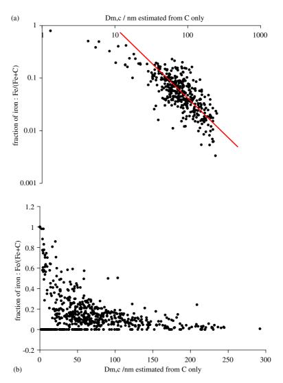
Fig. 14. Size dependence of iron fraction in diesel exhaust particles for the case of low-Fe doping: (a)  $0\,\mathrm{W}$  load, and (b)  $6\,\mathrm{kW}$  load. (Note: solid line through data shows  $D_{\mathrm{m.c}}^{1.31}$  dependence.)
