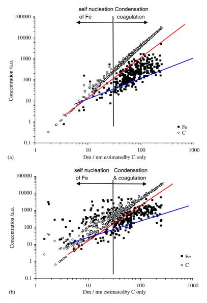
Fig. 11. Size dependence of iron and carbon fractions in diesel exhaust particles for the case of high-Fe doping: (a) 0 W load, and (b) 6 kW load. (Note that upper line shows  $D_{\rm m,c}^2$  while lower line shows  $D_{\rm m,c}^1$ .)
