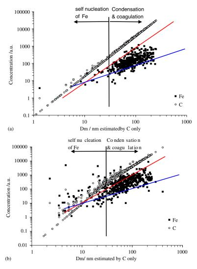
Fig. 12. Size dependence of iron and carbon fractions in diesel exhaust particles for the case of low-Fe doping: (a)  $0 \, \text{W}$  load, and (b)  $6 \, \text{kW}$  load. (Note that upper line shows  $D_{\text{m,c}}^2$  while lower line shows  $D_{\text{m,c}}^1$ .)
