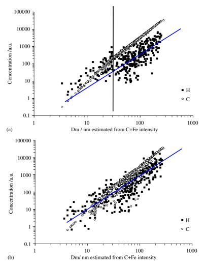
Fig. 10. Size dependence of carbon and hydrogen in diesel exhaust particles for the case of high-Fe doping: (a) 0 W load, and (b) 6 kW load. (Note: solid line through data shows  $D_{m,c}^2$  dependence of elemental concentration.)
