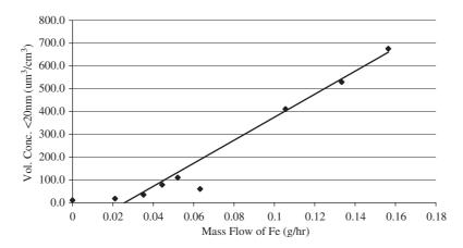
Fig. 6. Total volume of nuclei-mode particles (< 20 nm) as a function of Fe feed rate.
