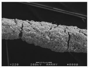
Figure 1. SEM image of T-Jump probe coated with Al/CuO nanocomposite mixture.
