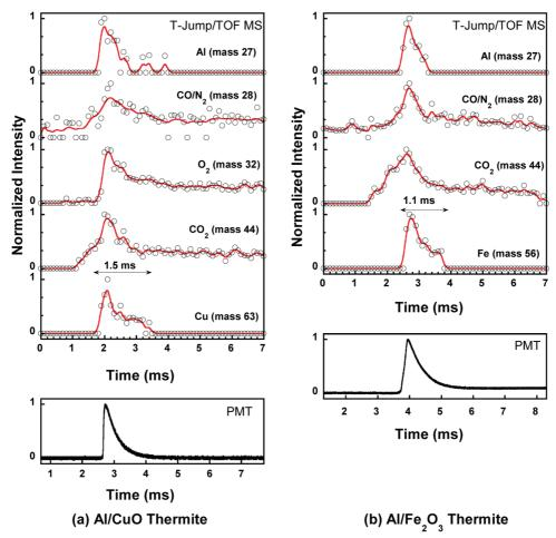
Figure 8. Normalized peak intensities as function of reaction time for reaction species observed in (a) Al/CuO and (b) Al/Fe<sub>2</sub>O<sub>3</sub> reactions; the bottom plots are optical signal measured from separated experiments.
