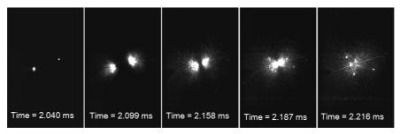
Figure 3. Selected images for a Al/CuO nanocomposite reaction recorded by a high-speed camera.
