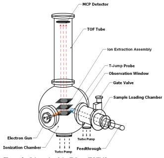
Figure 2. Schematic of the T-Jump/TOFMS.
