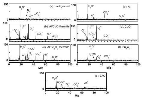
Figure 5. Detailed views of selected mass spectra obtained from T-Jump experiments. (a) Background, (b) Al/CuO mixture, (c) Al/Fe<sub>2</sub>O<sub>3</sub> mixture, (d) Al particles, (e) CuO particles, (f) Fe<sub>2</sub>O<sub>3</sub> particles, (g) ZnO particles.
