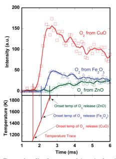
**Figure 6.** Temporal profile of oxygen peak intensity from heating of CuO, Fe<sub>2</sub>O<sub>3</sub>, and ZnO nanoparticles.
