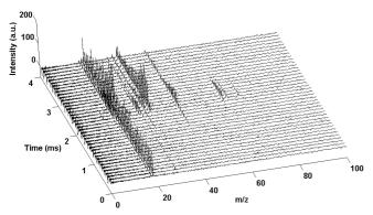
Figure 4. Time-resolved mass spectra obtained from Al/CuO nanocomposite reaction. Sample heating start at t = 0.
